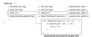
Figure 6: Example of using type mapping DSL in ConnectorX, with illustration of simplified generated code.
