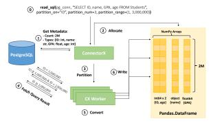
Figure 4: Workflow of ConnectorX.
